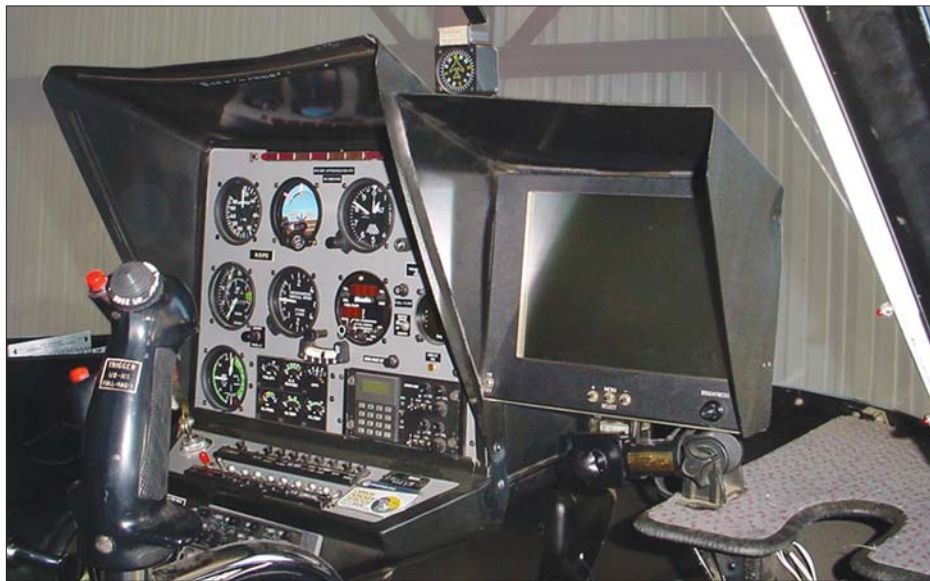
F28F with a Field Installation FLIR Installed
